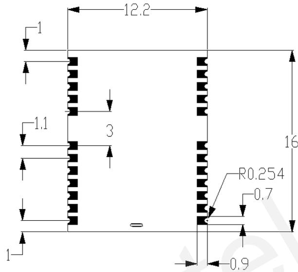
**Figure 18: Bottom Dimension (Unit: mm)**
