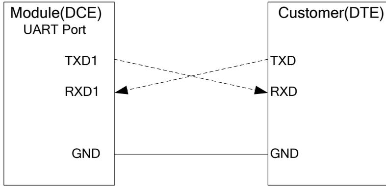
**Figure 11: Connection of Serial Interfaces**
