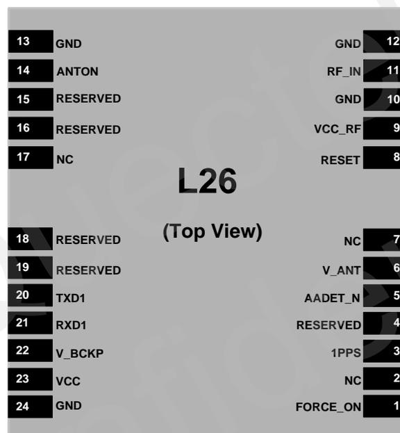
Figure 2: Pin Assignment
