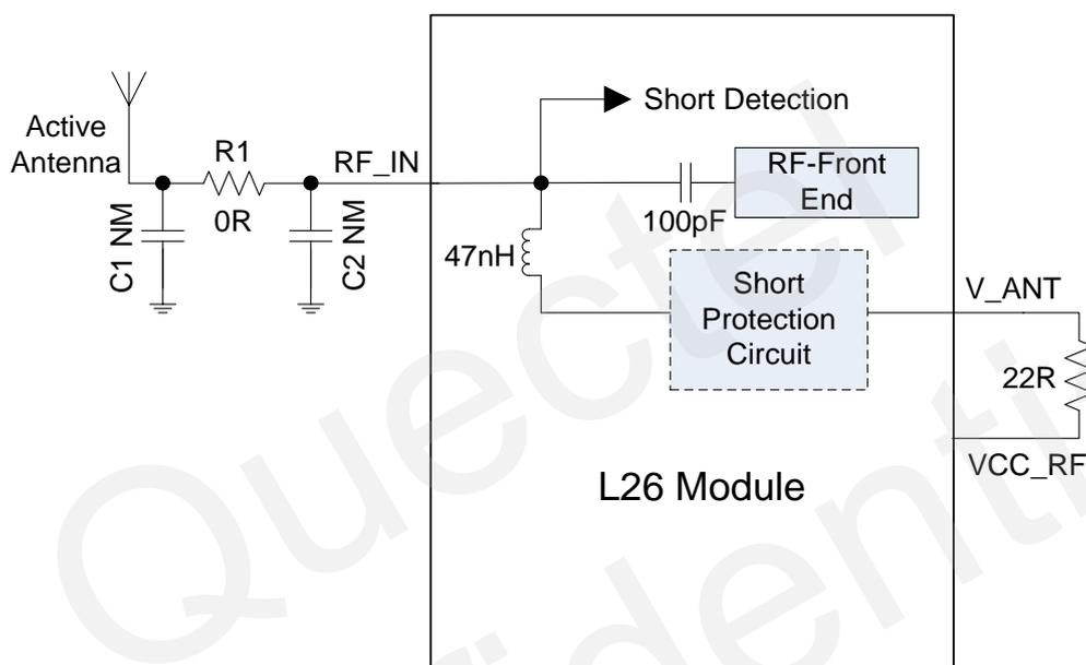
**Figure 14: Active Antenna Reference Design with Short Protection**
