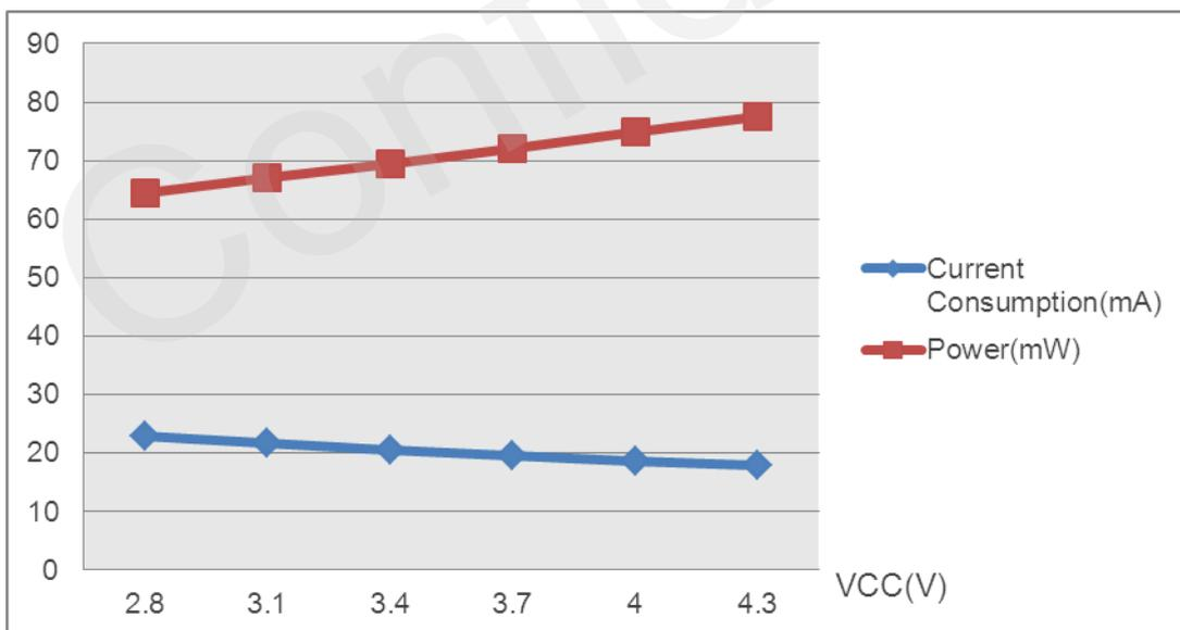
**Figure 4: Power and Current Consumption versus VCC**
