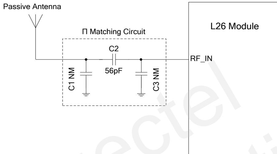
**Figure 13: Reference Design with Passive Antenna**
