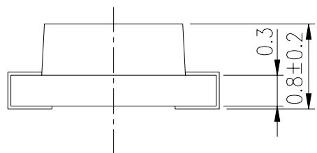
**For reflow soldering (propose)**
